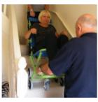
4. Using a suitable method transfer a 5. Using 2 people with 1 at the front and 1 at the back, move forward over the for security and comfort, place the top step, allowing the 3 rotating wheels persons feet on the footrest if required. to balance, lower the chair and Fasten the safety belt and move to the continue down each step. Once you are at ground level move to a place of safety.
