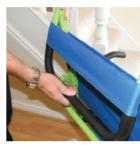
2. Remove safety pins on each side and fold away handle extension.
